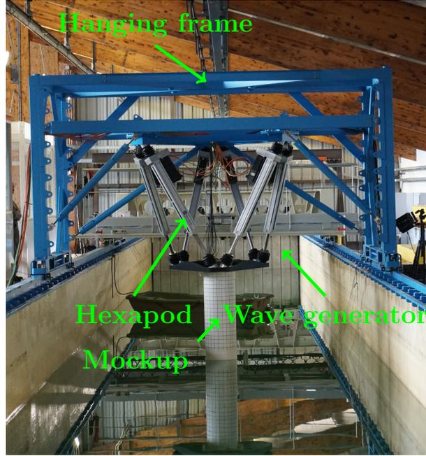
FIGURE 1 – Overview of the mockup mounted over the flume
