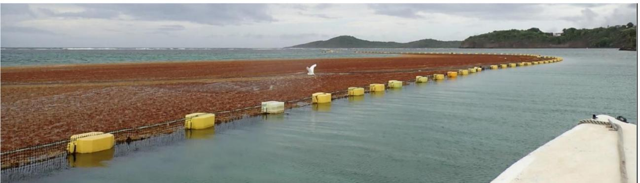
Figure 3. Floating barrier for algae containment or deviation FILET DROM©, each section is 50 m long, until 2 m height, and is moored on bloc, anchor or pile.
