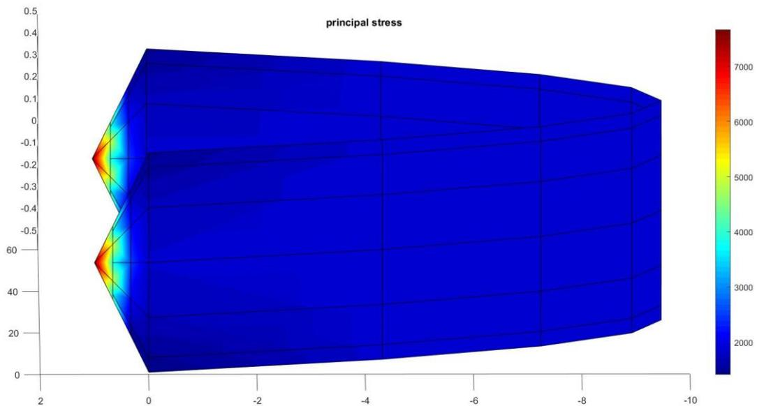
Figure 7. Stressmap (N.m-1) in the barrier, velocity 0.35 m.s-1.
