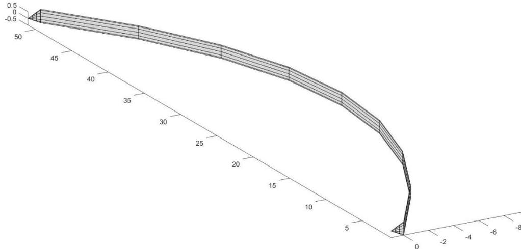
Figure 6. Finite-element mesh, parabolic initial geometry, 158 nodes, 156 elements, flattened cylinder with two cones rotated at 90° giving the mooring devices. X-longitudinal Y-upstream Z-vertical.
